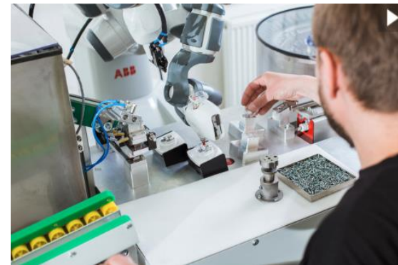
YuMi and human worker jointly assemble sockets at an electronics factory
