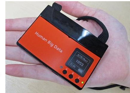
Wearable nametag for measuring the actions of people within an organization.
