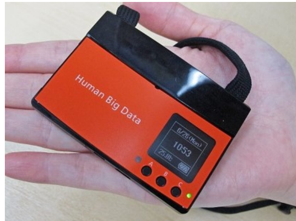
Wearable nametag for measuring the actions of people within an organization.
